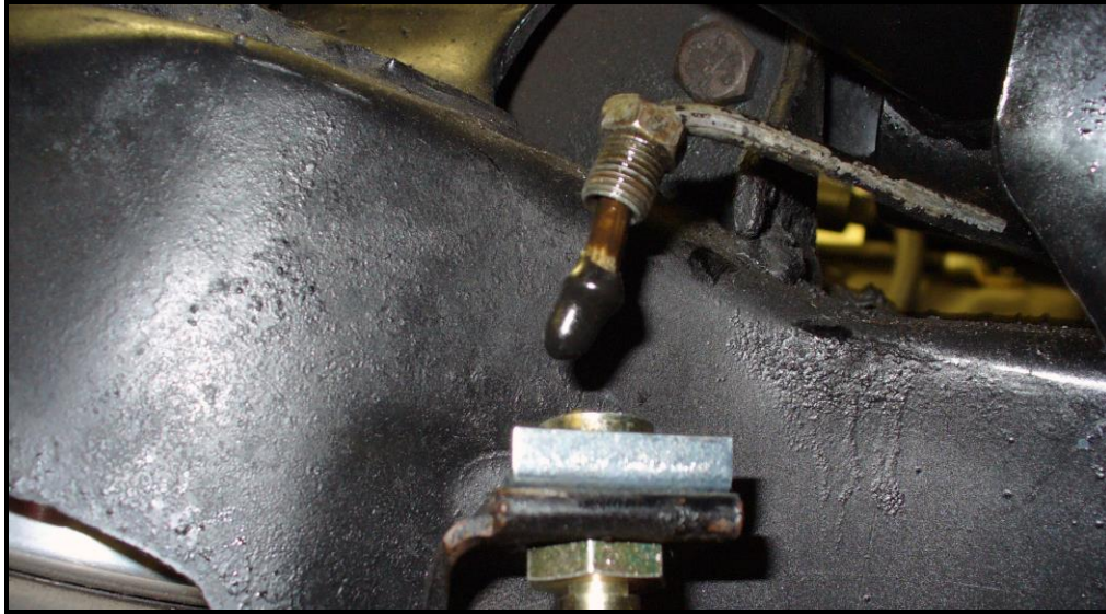
Hose lock location and vinyl cap installed
