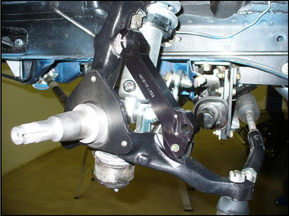
Left bracket installed, caliper to rear of spindle pin
