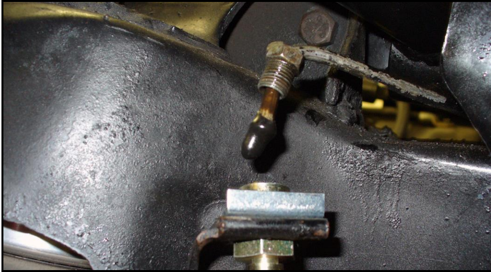
Hose lock location and vinyl cap installed
