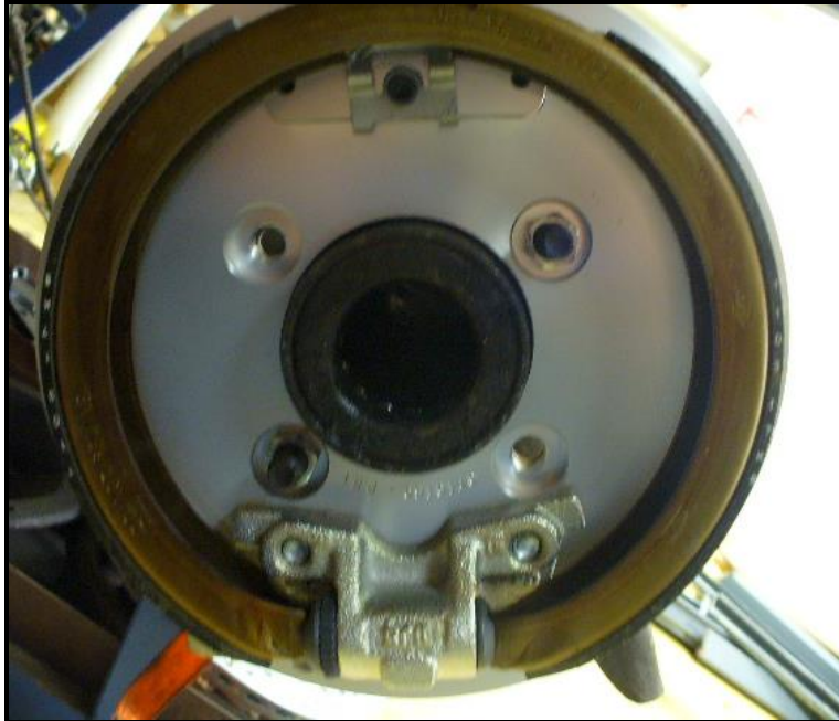
Park brake assembly correctly installed
