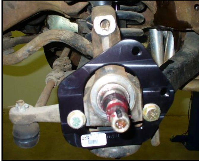
Left bracket installed, caliper to rear of spindle pin
