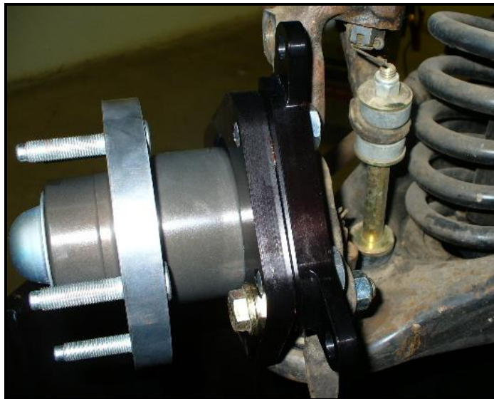
Intermediate bracket installed Part number engraved on bracket faces outward
