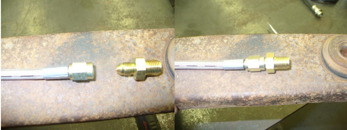
Install adaptor into AN fitting on hose and torque 15-20 ft-lbs.
