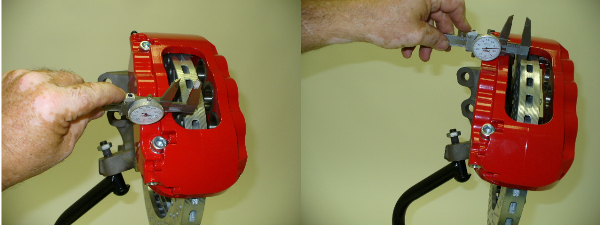
Measure top and bottom, inboard and outboard.
