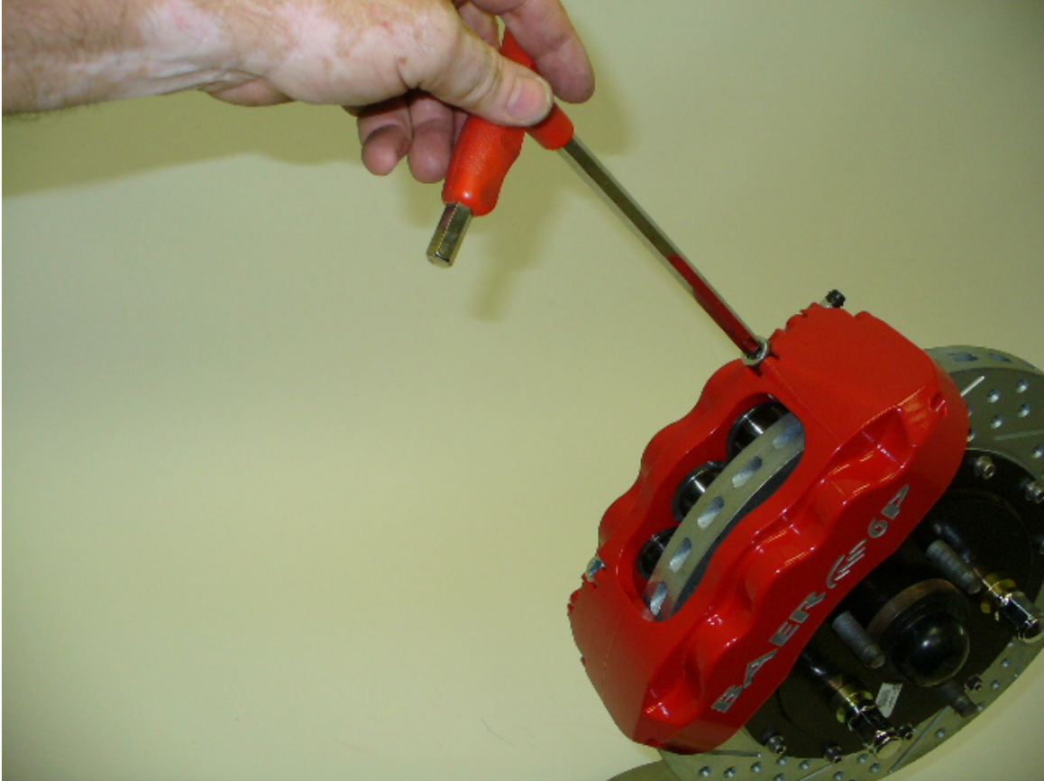
Caliper installed without pads.
