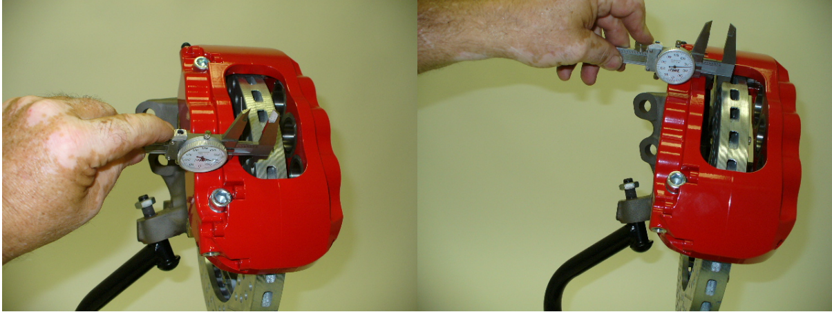
Measure top and bottom, inboard and outboard.
