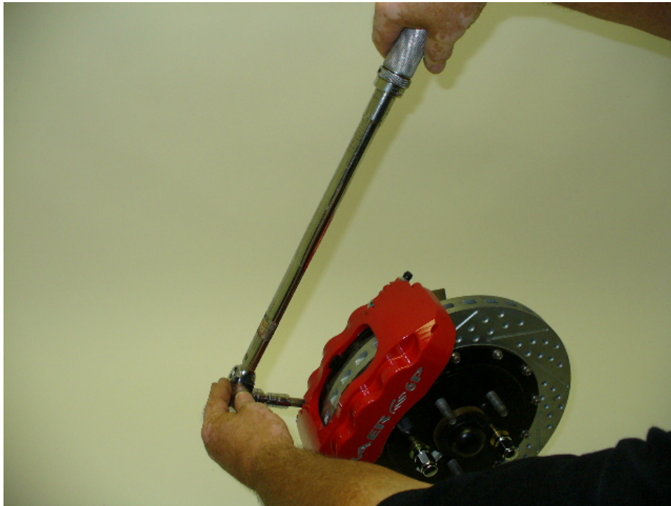
Torque caliper bolts to 85 ft-lbs.
