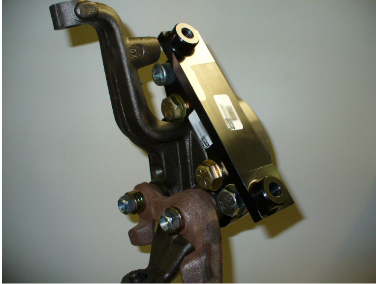
Radial mount bracket installed.
