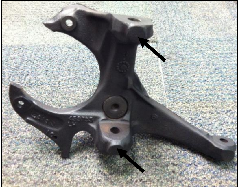
Figure 2: Strike here to dislodge ball joints
