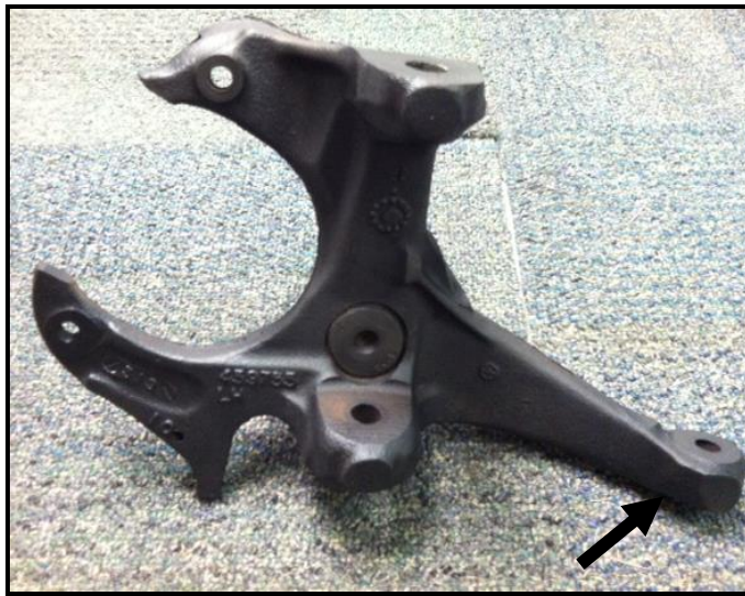
Figure 1: Strike tie rod end boss here with large hammer
