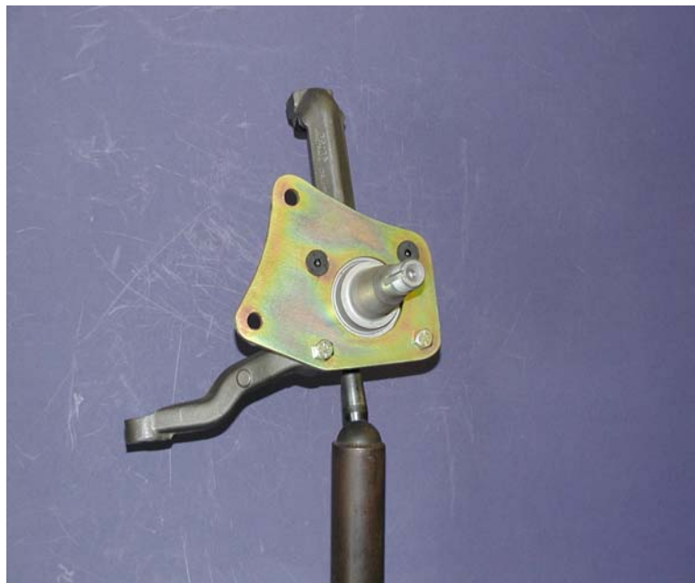
Right side intermediate bracket installed.
