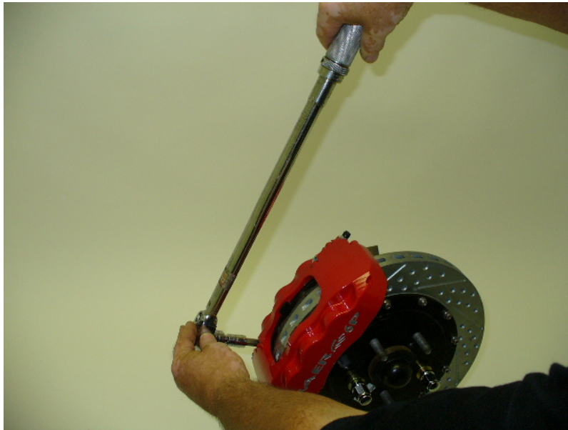
Torque allen caliper bolts to 85 ft-lbs.
