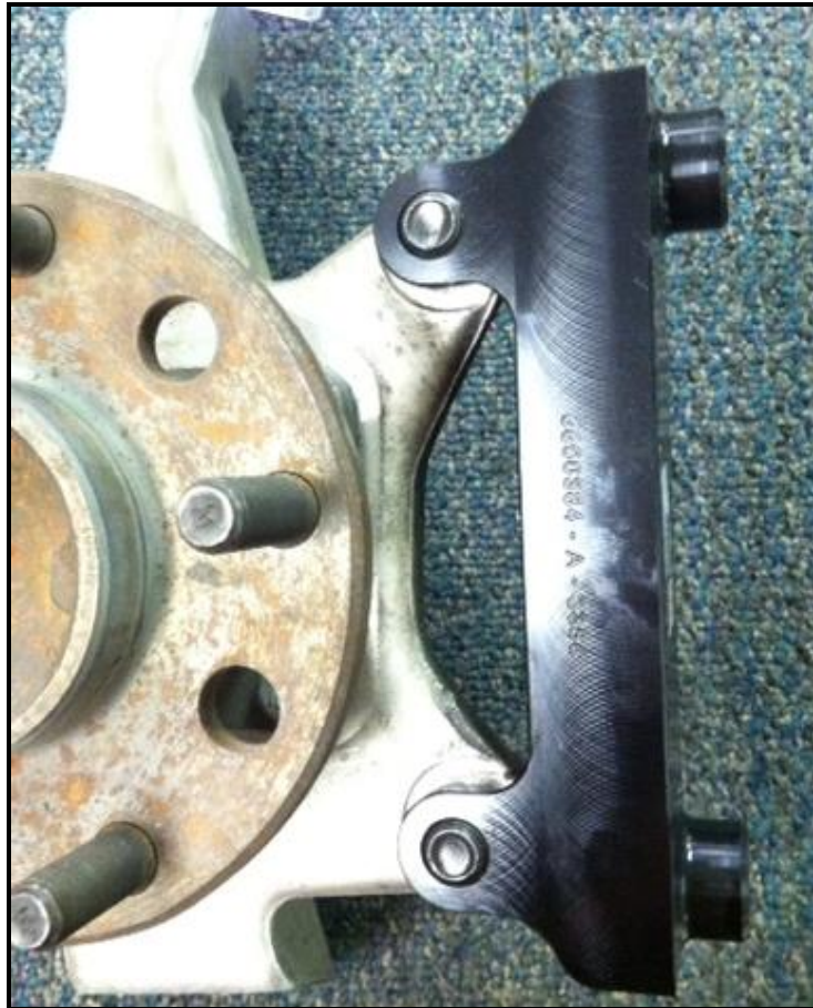
Figure 1: Base bracket installed onto spindle
