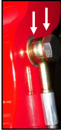
Figure 5: Installation of hose and washers
