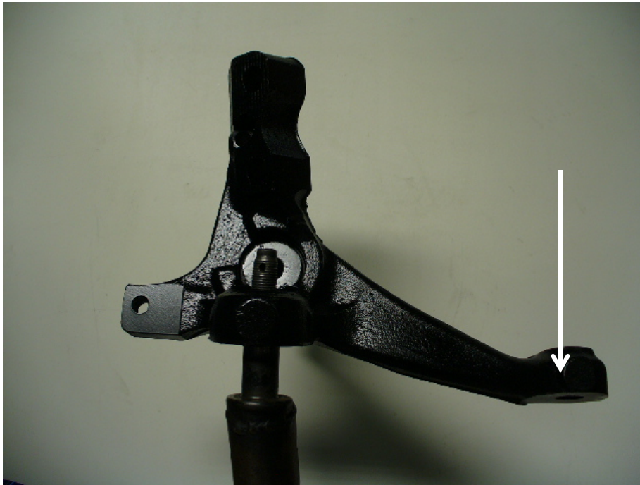
Strike tie rod end boss here with large hammer.
