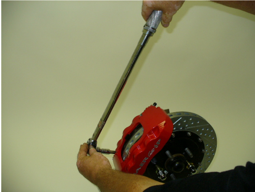
Torque allen bolts to 85 ft-lbs.
