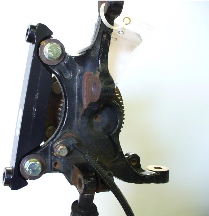
Radial mount bracket installed on spindle
