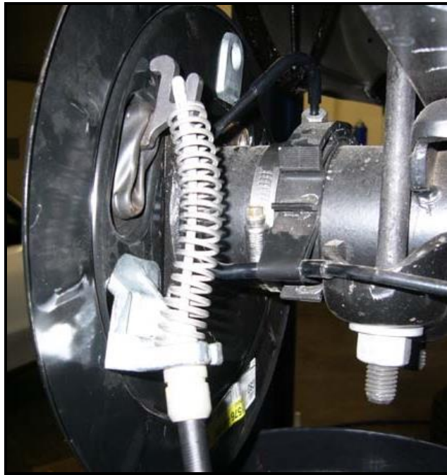
Figure 3: Left park brake assembly installed with cable attached
