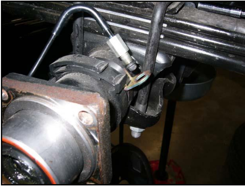
Figure 2: Right (passenger) side hardline retainer position
