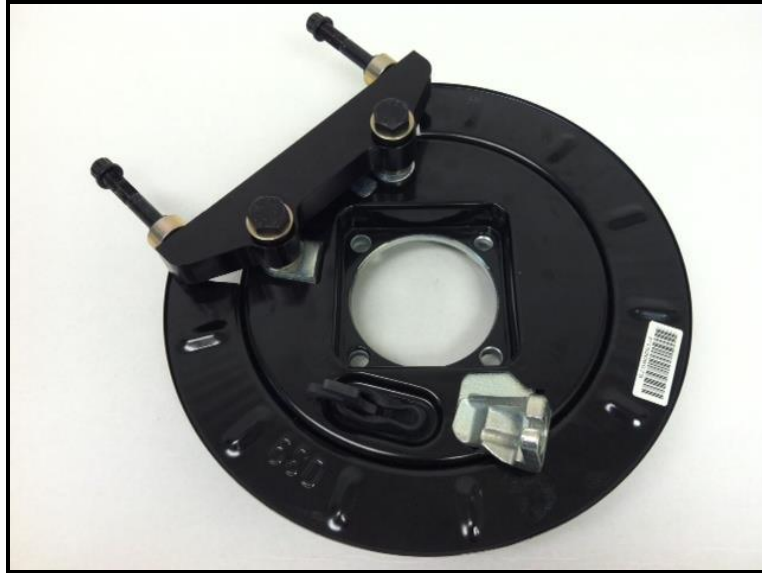
Figure 6: Inboard view of park brake assembly
