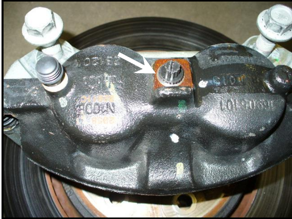
Side mount fluid inlet caliper 2010-2013 model year
