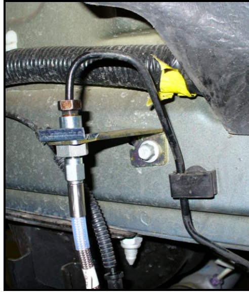
Figure 5: Brake hose attached to hardline
