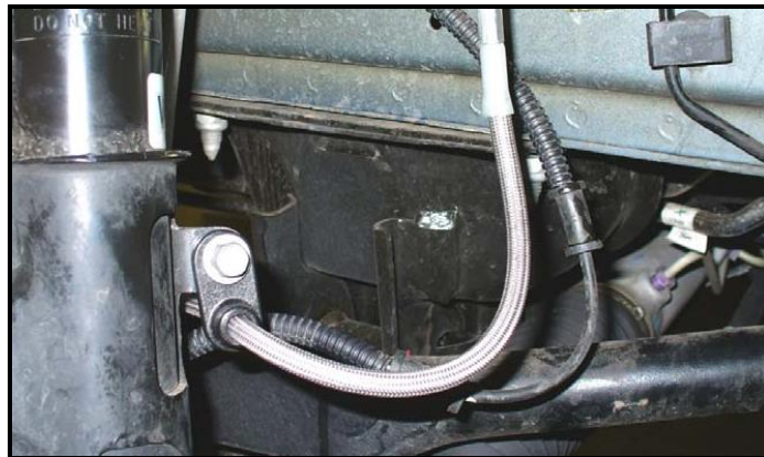
Figure 6: Brake hose attached to the plastic hose tab
