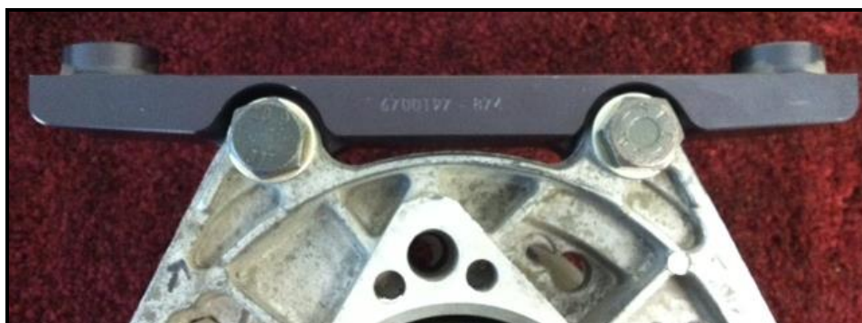
Base bracket mounted to outboard face of hub
