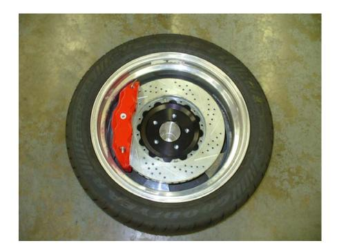
• When installing rotors on any Baer Products be sure to follow the direction of rotation indicated on
