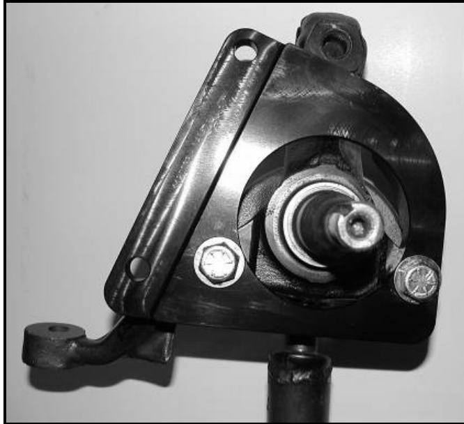
Figure 2: Rear Steer spindle shown with base bracket
