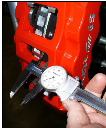
Figure 3: Measuring distance from rotor to caliper body
