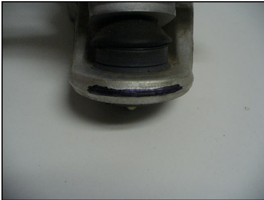
Figure 1: Area which may need trimming for rotor clearance
