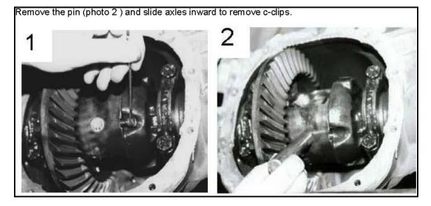
Remove the axles, taking care not to damage the seals. This is a good time to inspect the seals, axles and bearings, replacing as necessary. Also, measure the outside diameter of the axle flange. To properly seat in the rotor, the flange diameter can not exceed 5.9". If yours is larger, a machine shop can turn these down for proper fit.
