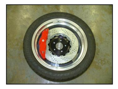
When installing new Baer rotors, be sure to follow the direction of rotation indicated on the rotor
