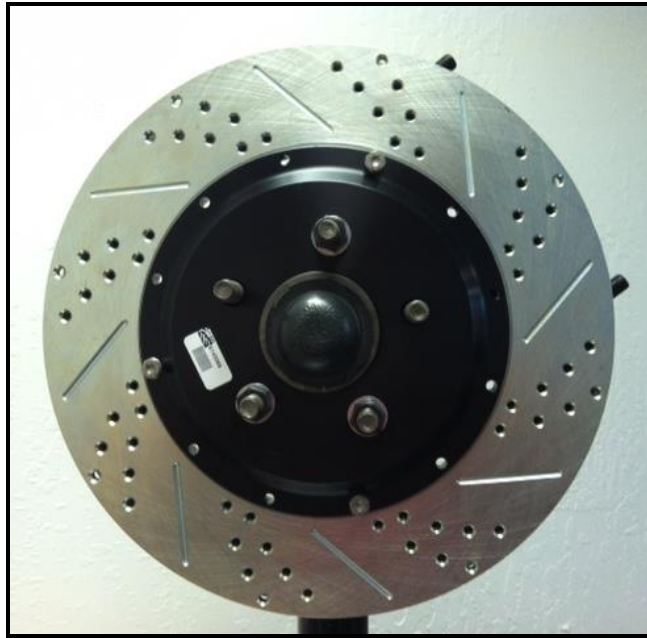
Figure 4: Rotor installed with lug nuts and washers
