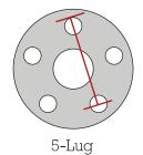
Back of hole to the center of the second bolt hole
