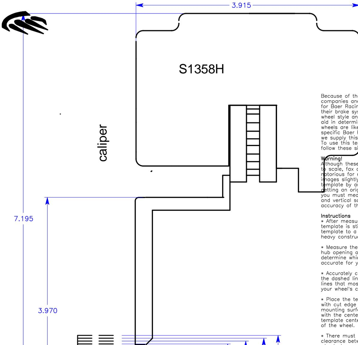
Because of the abundance of wheel companies and styles, it is impossible for Baer Racing to guarantee fit of their brake systems into a specific wheel style and/or manufacturer. To aid in determining for yourself if your wheels are likely to fit around a specific Baer Racing brake upgrade, we supply this brake system template. To use this template to determine fit, follow these simple instructions.
