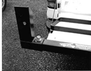
place Backrack c/w Railmount Bracket on to Rail Plate and secure to Stake Pocket Bolt
