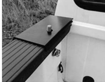
attach Railmount Bracket to Backrack Frame
