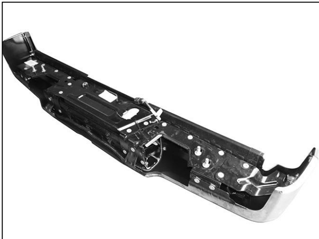
(Fig 7) Remove sensors, wire harness, license plate lights and trailer plug if equipped
