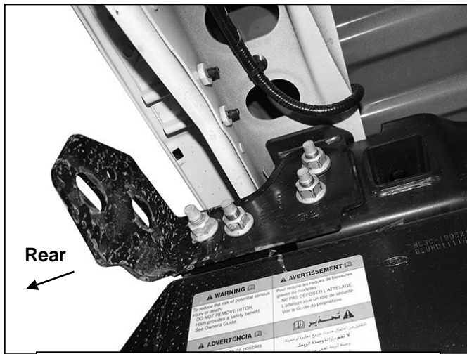
(Fig 3) Remove bumper bracket from frame
