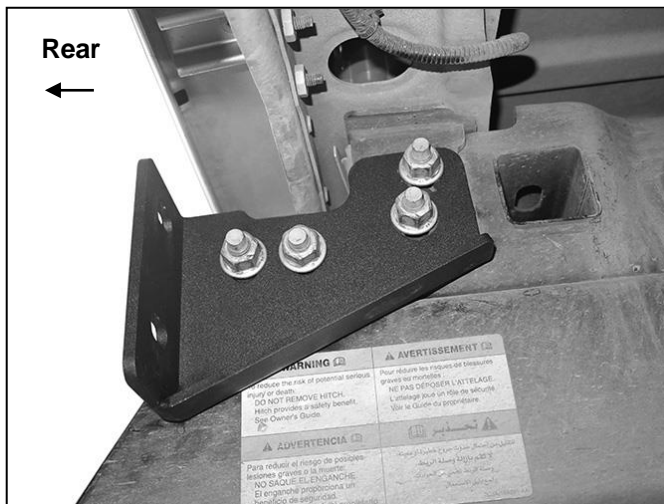
(Fig 5) Reuse factory hardware to attach the passenger/right Frame Mounting Bracket
