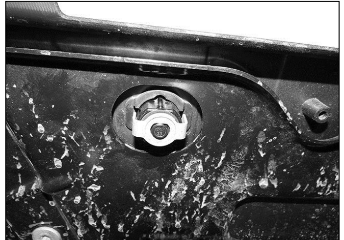
(Fig 4) Remove sensors, wire harness, trailer plug and spare tire access lock (pictured) if equipped
