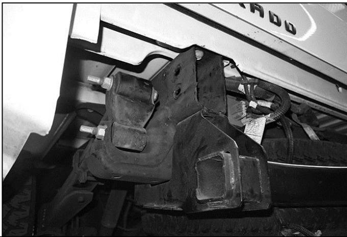
(Fig 3) End of frame once factory bumper is removed
