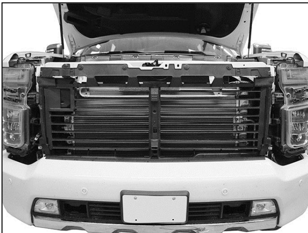
(Fig 7) Grille and fascia removed
