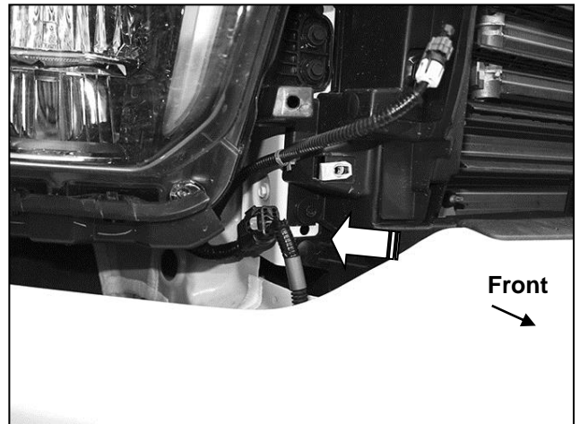
(Fig 6) Disconnect all wire harnesses leading to front bumper
