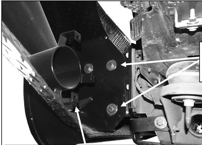
(Fig 13) Attach factory fog light to mounting tabs
