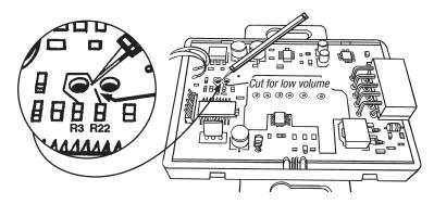
**Note:** If the chime volume of the GMRC-04 is too loud you will need to remove the cover and cut the solder connection where the arrow points to on the circuit board (between the holes on the board).
