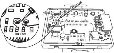
**Note:** If the chime volume of the GMRC-01 is too loud you will need to remove the cover and cut the solder connection where the arrow points to on the circuit board (between the holes on the board).
