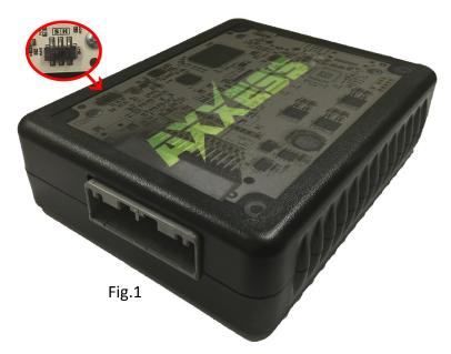
Switch is preset in the correct position for most installations, only in some cases you may need to adjust the switch position, or if image is not displayed correctly on the screen.
