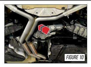
It is crucial to install each section and Accu-Seal clamp correctly to prevent loose joints and exhaust leaks between the tubing connections.
