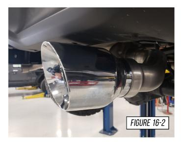
Check for proper clearance and tighten all clamps in the system to at least 60 ft/lbs, as shown in **Figure 17**.
