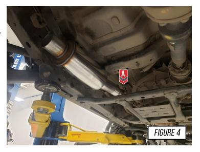
It is crucial to install each section and exhaust band clamps correctly to prevent loose joints, exhaust leaks and rattles.
