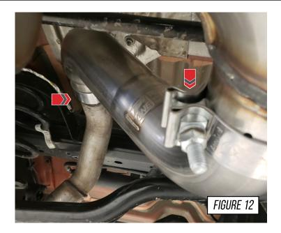
Install the AWE driver (**D51**) and passenger (**D52**) side tubes, with the supplied clamps, as shown in **Figure 13-1** and **Figure 13-2**.
