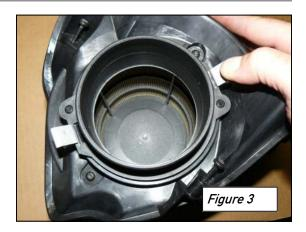
Install the AWE Tuning S-FLO Filter into the airbox lid by lining up the rubber bosses on the filter with the openings in the airbox lid.
