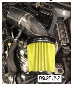
Align the silicone flex hose and tighten the 2 hose clamps, as shown in **Figure 13**.
