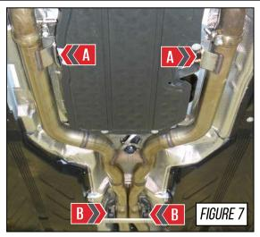
Move the rubber hangers from the OEM H-Pipe and place them onto the AWE Tuning H-Pipe, at **Arrows B** in **Figure 7**.
