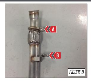
With the front tube sections installed, snug the OEM V-band clamps into place, be sure to allow for adjustment. Shown by **Arrows A** in **Figure 9**.
