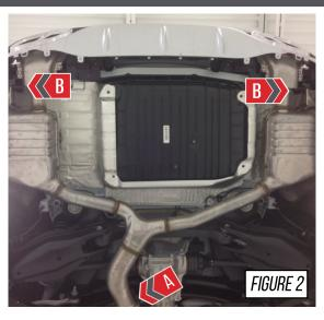
Remove the six (6) 10mm plastic nuts and four (4) 8mm bolts that are along the tunnel, examples shown by **Arrows A** that surround the chassis brace; shown by **Arrow B** in **Figure 3**.
