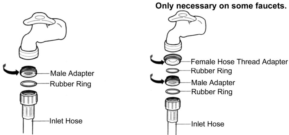
**If water leaks from faucet connection or washer connection, turn off water and tighten fully using a wrench. Be careful not to over tighten and damage water connection. Turn on water supply and make sure no leaks are present.**
