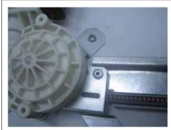
1. Drill rivet located at bottom of track. Drill bit needs to be larger than a 1/4 inch.
