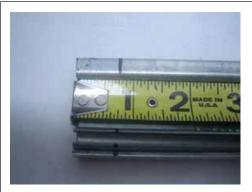
4. On the bottom of the track, mark 3/4 of an inch.
