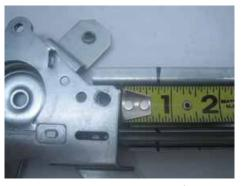
3a. Make a mark on the track from top of motor mount to 3/4 of an inch.
