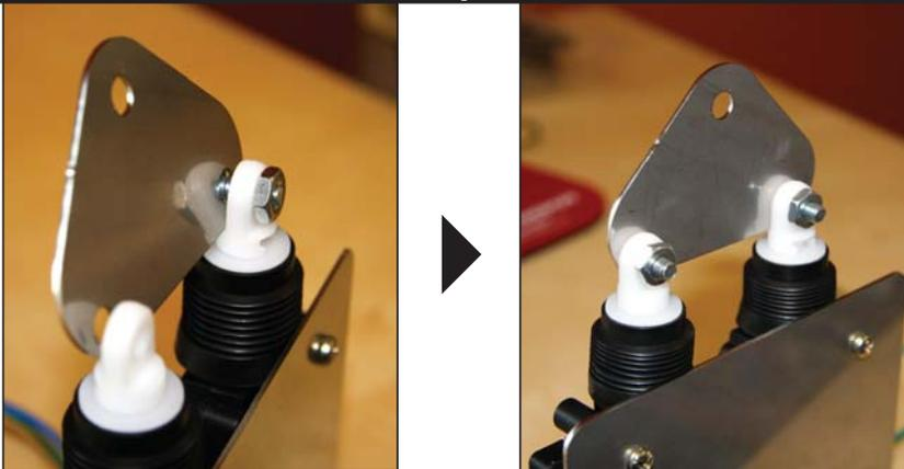
Take the triangle mount and the 1/2" nut & bolt and secure it to the actuators's arm (the white fixture).
