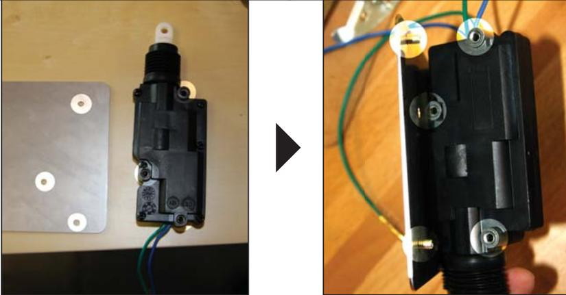
Align the actuator mount screw holes with the actuator's. Secure the actuator to the mount using the 1/4" screws. *\*Special Note* - you might want to pre thread the actuator screw holes before attaching it to the mount for easier installation.
