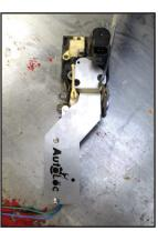
Make sure the latch is in the unlocked position. Slide the bracket over the same lever, then line up the three holes on the bracket with the three holes on the latch.
