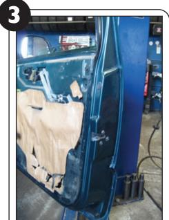
Using a pick or similar tool, un-snap the plastic retaining clip that holds the rod to the back of the inside handle. Be careful not to damage the rod; you will reuse it.
