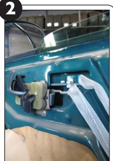
Remove the door panel and 3 torque screws that hold the latch. For most GM vehicles, screw size is T30.
