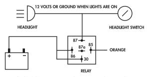
NOTE: If parking lights are negative trigger, then connect 30 to chassis ground.
