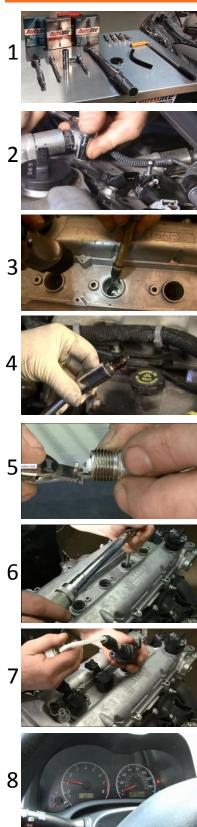
Replacing spark plugs can be a simple job, if you take things one step at a time. Here's a general guide to the proper procedures. **Read the entire process first!**
