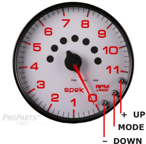
The SPEK™ RPM Tachometer can be programmed to monitor, display and control precision engines to meet the customer's expectations and surpass industry standards. The following programming instructions are divided in to two sections. please select only that section that meets your requirements.
