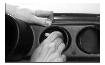
2. Install mounting brackets on pod using enclosed Allen screws. Use a 5/32" Allen Wrench.
