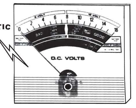
Mix a solution of 1 part liquid dish soap with 4 parts water and wipe on the meter cover.
